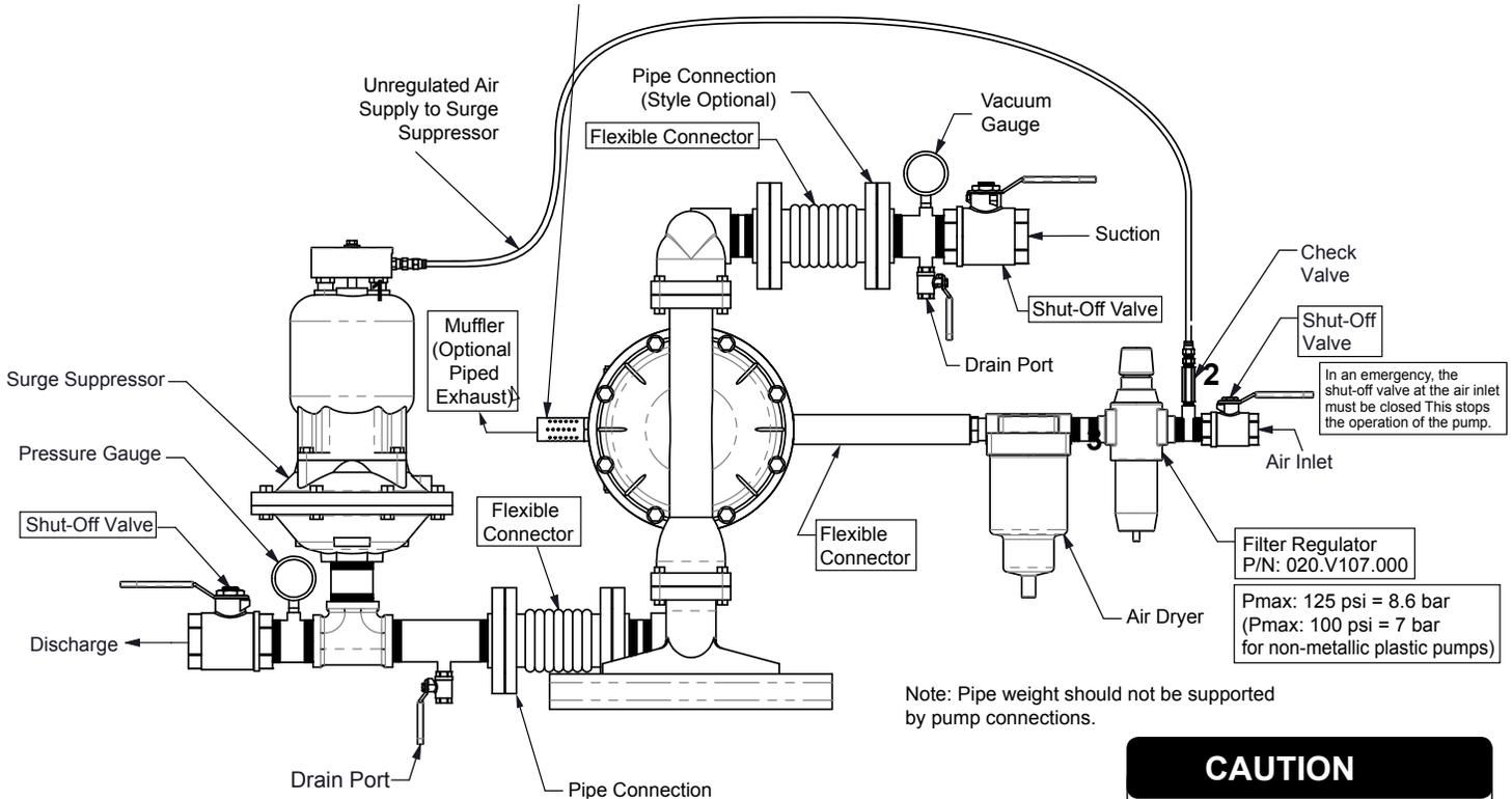
**Note:** Surge Suppressor and Piping must be supported after the flexible connection.
